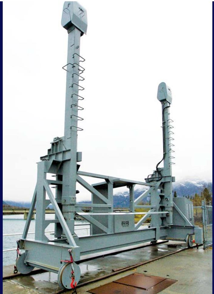
The electric motor (propane engine optional), pump, oil reservoir and control bank will be contained in their own lockable enclosure of 12 Ga. material.
